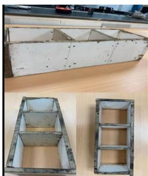
Figure 1 - Improved molder for multi-nutrient lick block production
