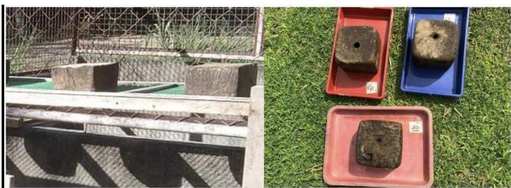
Figure 2 - Sun drying of MNLB for 30 to 35 days
